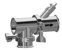
If the try-clamp version is used, no tools are required. Try-clamp fasteners should only be hand tightened without using any tools
